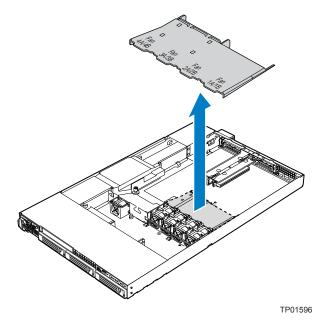
Figure 13. Removing the Processor Air Duct
